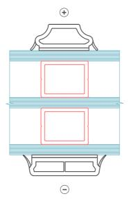
Combinated PVC bars Glued on both sides: Classic 22mm inside Standard 27mm outside +Duplex 3 layer glass
