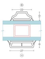
Combinated PVC bars Glued on both sides: Classic 22mm inside Standard 27mm outside +Duplex 2 layer glass
