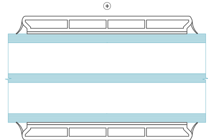
⊖ Standard PVC bars Glued on both sides 77mm 3 layer glass
