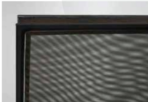
Fig. 21 Moiré effect in insulating glass unit.
