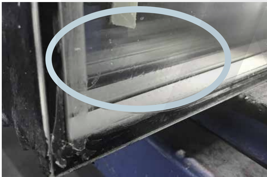
Fig. 28 Delamination of PVB film due to chemical incompatibility
