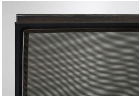
Fig. 21 Moiré effect in insulating glass unit.
